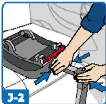
Squeeze together the isofix adjustment buttons located on either side of the support leg at the front of the car seat base and pull the support leg towards the seat base to extend the isofix attachment points.
