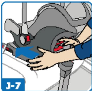
Push the baby seat firmly against the backrest to lock it into the isofix fittings. Check the indicator light to confirm your baby seat is correctly installed.
