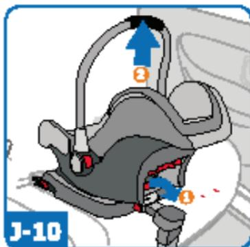
Press the release button and pull the handle upwards to remove the car seat from the base.
