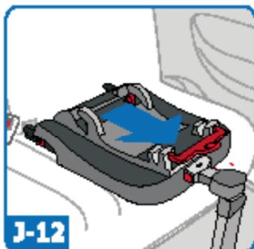
Pull the car seat base away from the back seat to release from the vehicle.
