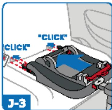
Line the isofix attachment points with the isofix latches in the vehicle seat and push the isofix points into the isofix latches until you hear a "click".
