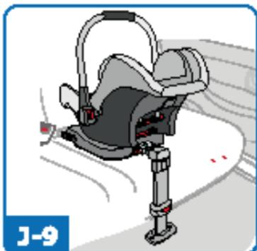
The rearward-facing baby seat is fitted correctly on your car seat.
