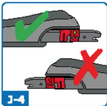
When the isofix points are correctly attached the isofix connection indicators will turn green.
