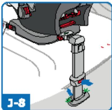
Adjust the leg to the right height by pressing this button. Make sure the leg is stable against the floor and lock it firmly into position and check the indicator light (it will be green).
