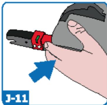
Unlock the isofix points by pulling the latches towards the front of the vehicle seat.
